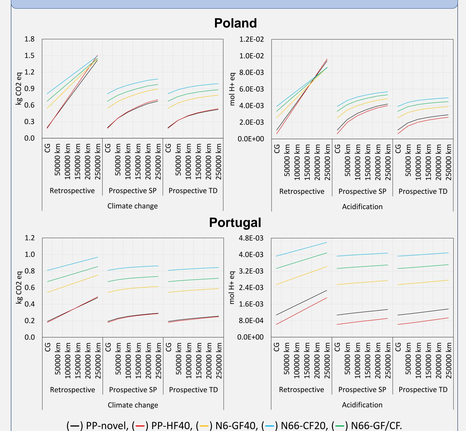
Figure 4. Cradle-to-use impacts of one automobile interior door handle throughout a lifetime distance of 250 000 km in 15 years.
